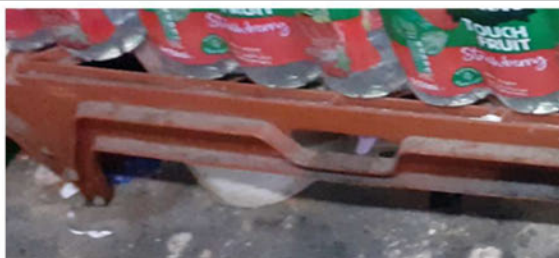
Pallets too close to floor to allow cleaning & also inspection for pests.
